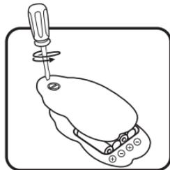
4. Install 2 new 'AAA' (LR03/AM-4) batteries into the remote control following the diagram inside the battery box.
