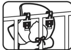
3. Pull slightly on the unit to make sure both straps have been securely fastened. The unit should be snug against the cot rail. Please check the unit frequently to ensure it is still secure.
